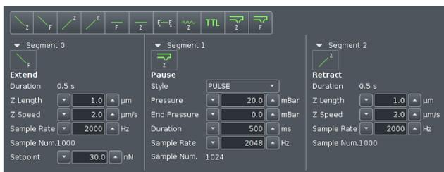
**Fig. 4: Integration of the FluidFM functionality in the RampDesigner.** Synchronisation of AFM and pressure adjustments
