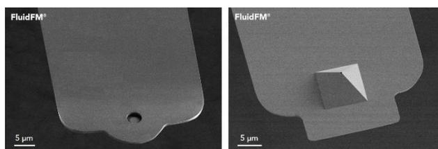
**Fig. 2: Examples of FluidFM probe types.** FluidFM micropipette with a 4 µm aperture (left), and FluidFM nanopipette equipped with a pyramidal tip with a 300 nm aperture (right). Image courtesy of Cytosurge AG.
